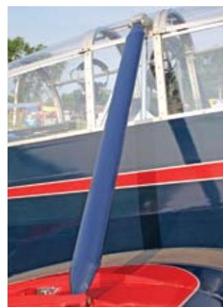
**Closeup view of the inboard strut.**
