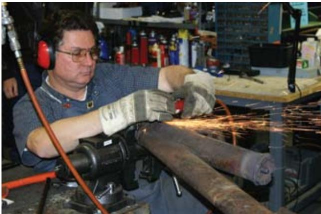
**Addison works on the massive landing gear. All of the parts of this biplane are big!**
