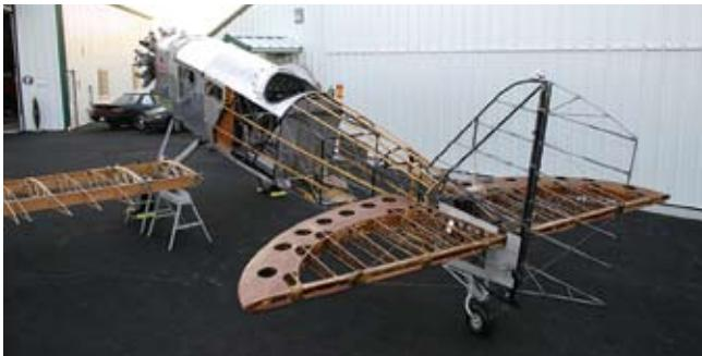
The airframe is nearly complete. Addison refers to the Boeing construction as “hobbyist” in the sense that since it uses few castings or forgings, the airplane can be hand built. Given its size, that means there were a lot of hands! Sixty-one volunteers were logged by the Pembertons, 10 of whom hardly ever missed a Wednesday night restoration session.
