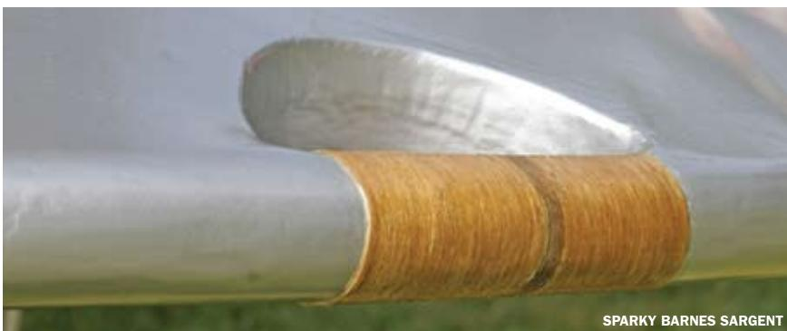
**The wingtip's hand grip is neatly trimmed with cord to reduce wear and give a ground handler a good grip.**
