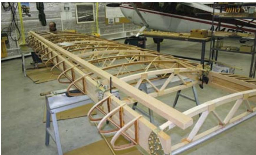
One of the four wing panels built for the Boeing.
