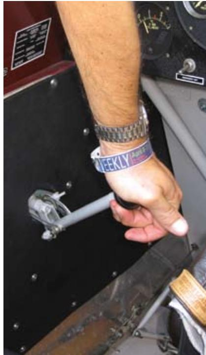
**Close-up view of the throttle/brake lever.**
