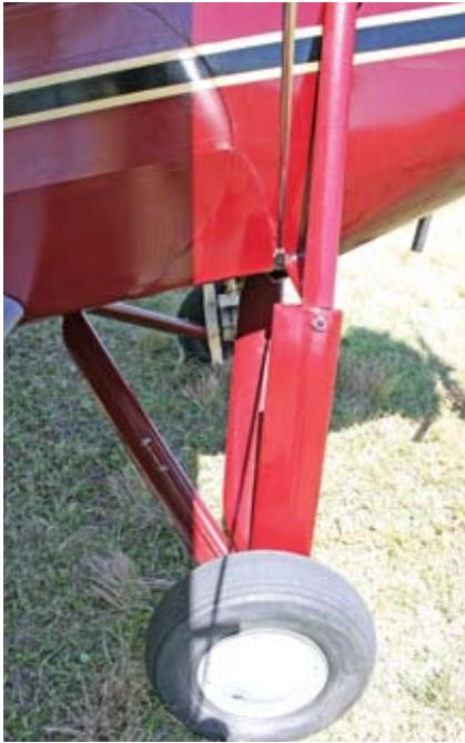
**Close-up view of the Waco's outrigger gear.**
