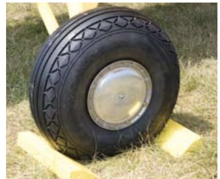
**These two shots show the Desser Aero Classic tires and Aeronca embossed wheel covers. On this Champ, Van Sickle brakes were used. Due to supplier shortages during the years following WW-II, Champs and Chiefs were delivered with either Goodyear disc or Van Sickle drum brakes.**
