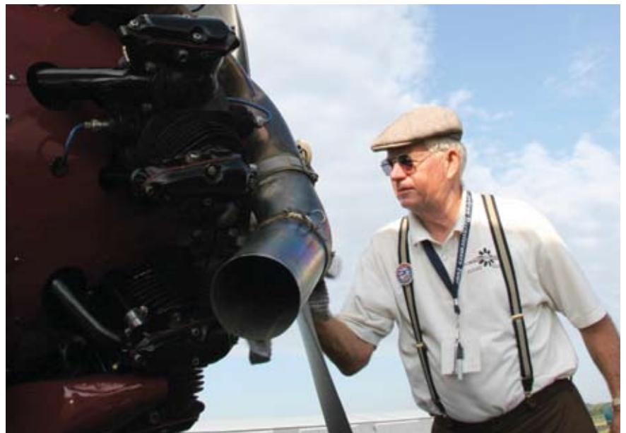
**Bob is checking the integrity of the Hamilton Standard prop during the American Barnstormers Air Tour 2006. The installation of a Wright R-760-8 engine required a supplemental type certificate that proved quite frustrating to obtain, even with the help of the original designer of the plane.**
