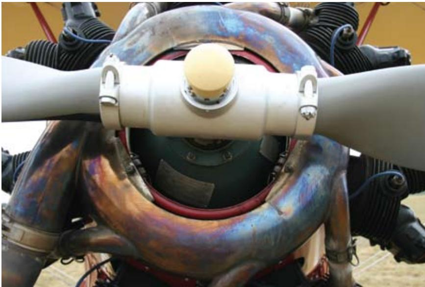
**Over the years, the exhaust collector had oxidized to acquire a pretty impressive array of colors, as depicted here.**
