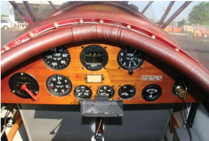
**The instrument panel of the Command-Aire is classic, and the instruments well-laid-out. The only modern addition is the GPS mount in the center of the panel.**
