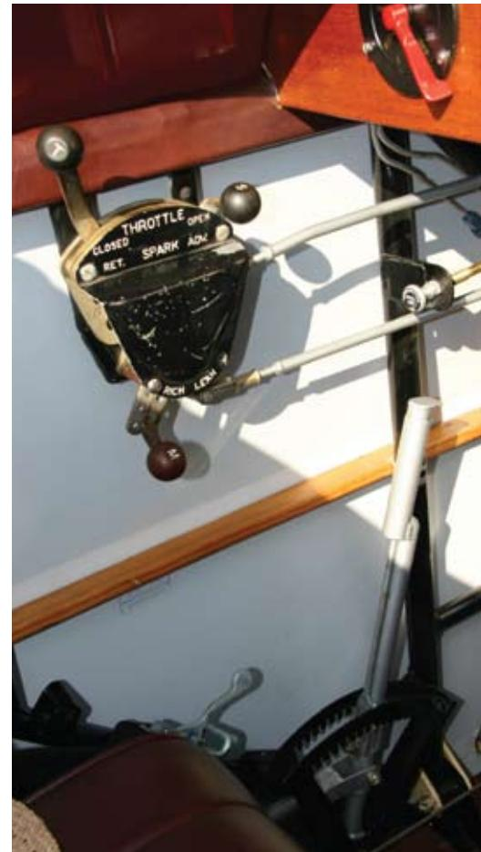
**One special feature of the Command-Aire is the ground- and air-adjustable tail incidence. The big lever seen in this picture allows it to be adjusted.**
